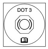
The brake master cylinder reservoir is filled with DOT-3 brake fluid. See *Engine Compartment Overview on page 5-12* for reservoir location and access.
